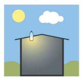
Putting a water-filled bottle in the hole collects more light because light rays travelling through denser-thanair material such as water change direction.
