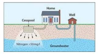
Figure 4. A schematic example of a cesspool. Source: groundstone.ca
