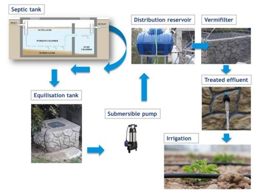
*Figure 15.* A schematic view of a demonstration vermifiltre built by WiSDOM association in a rural area of Moldova, at household level
