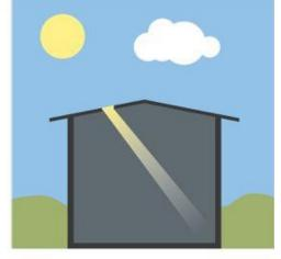
The water light bulb is simple and cheap. A 2-litre bottle is filled with clean water, plus about 10 millilitres of bleach in order to inhibit algae growth over time. The advantage to using solar water bulbs over simply cutting holes in the roof is that sunlight shining down a hole works like a spotlight, lighting only a small area within the room.
