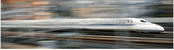
The high-speed train designed in Japan was inspired by the beak of a bird called kingfisher. In this way, it is possible to move forward with less friction and energy loss.
