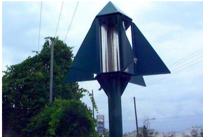
Figure 8. Air-turbo Vertical Axis Urban Wind Turbine by AIR-SUN ( www.air-sun.gr )
