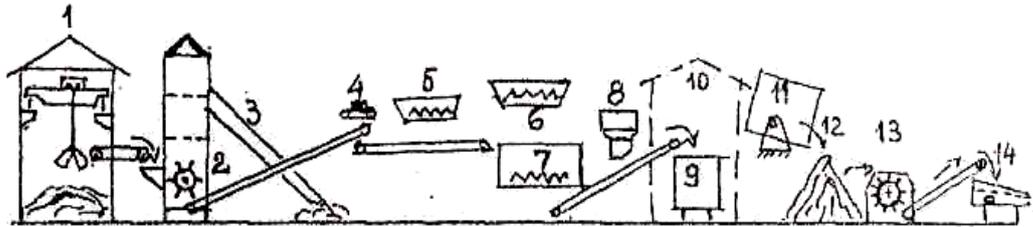
Picture 11-2: **Prat-Sofraïne procedure.** 1-bunker; 2- hammer crusher; 3- infrared separator; 4- magnetic separator; 5- compost dispenser; 6- domestic sludge dispenser; 7- mixer; 8- chemical reagents basin; 9- maturation cells; 10- cell storage bay; 11- cell discharge system by tilting; 12- posterior maturation prism; 13- grinding installation; 14- screen rotating drum.
