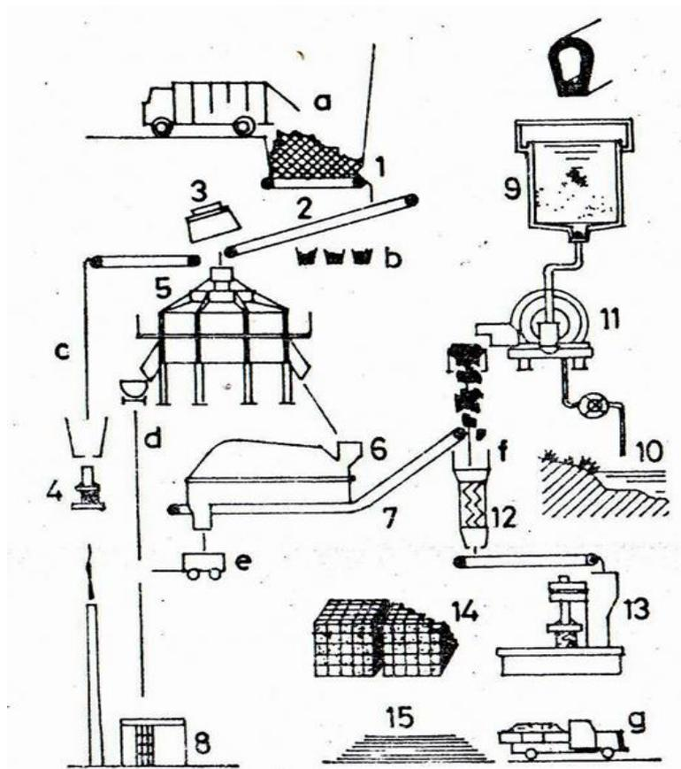
Picture 11-1: The technology process of Brikollare system: a-fresh waste; b-sorted materials; c-iron; d-sifted materials; f-dehydrated domestic sludge; g-compost.
